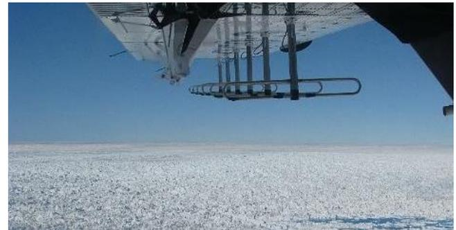
Figure 4 Folded dipole antennas under wing of Twin Otter
